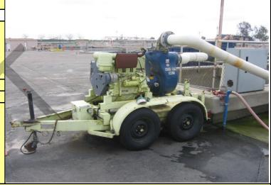
7. Justification & Useful Life: The 6" Gorman Rupp Trailer Mounted Trash Pump is over 30 years old. It has served the District well and has been used beyond its useful life. The new mounted trash pump will give us increased reliability and efficiency with the latest in new technology. The new mounted trash pump will have fewer unscheduled maintenance work orders and downtime for repairs and parts.
