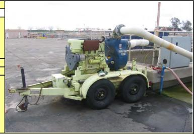
**7. Justification & Useful Life:** The 6" Gorman Rupp Trailer Mounted Trash Pump is over 30 years old. It has served the District well and has been used beyond its useful life. The new mounted trash pump will give us increased reliability and efficiency with the latest in new technology. The new mounted trash pump will have fewer unscheduled maintenance work orders and downtime for repairs and parts.
